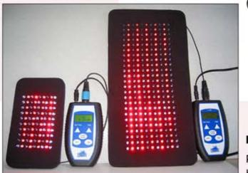
The units consist of two parts: the light pad, and a small microprocessor that controls the frequencies.
