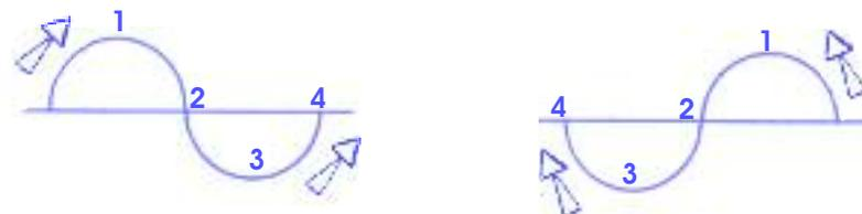
2. Fully polar rotational: alternating around the compass clockwise, then counterclockwise in sequence.
